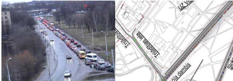
Fig. 6. Traffic flow video observation frames and modeling simulation results for the Raņķa dambis street
