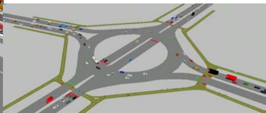
Figure 10. Traffic and pedestrian flows when central traffic island is cut along the high-street
