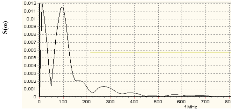
Fig. 3. Model spectrum of reflected signal on output of receiving antenna
